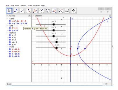
Standard and general equations of **parabola d**; p = 1, l = m = 2 (vertex (2,2))
